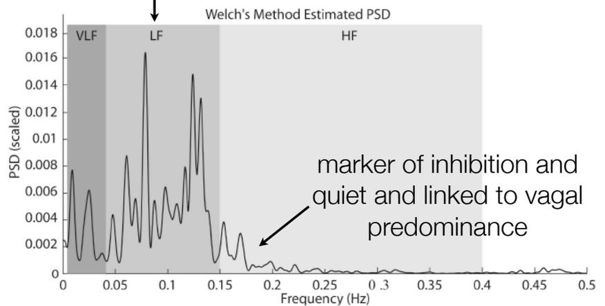
Fig. 8. Example of the heart rate spectrum in three subbands using the 1,024-point Fast Fourier transform.
